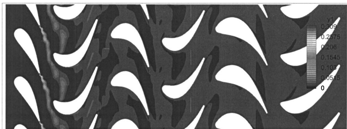
Fig. 13 Contour plots of methane mass fraction (case 1, first three stages)
