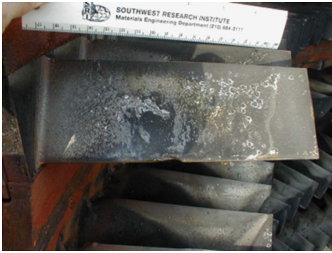
Fig. 8 Degraded compressor blade
