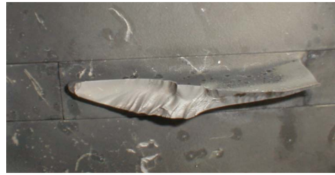
Fig. 3 Compressor blade failed due to flutter-induced high-cycle fatigue
